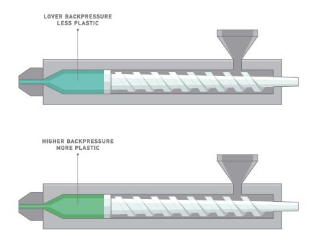
Back pressure is the pressure when taking place on front of the screw during screw retraction to prepare the next shot. Increasing it's values, collects more material on front of the screw, that's why if you don't change the injection speed strokes, your part weight would be heavier than before because of higher density taking place of the same volume in front of the screw.
