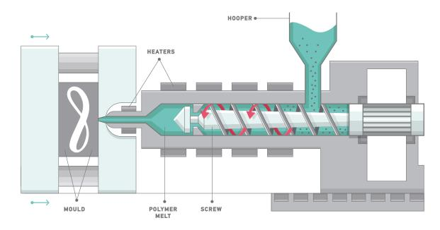
Injection molding machine is consist of two side, a clamping side and an injection side. The main purpose of the clamping side to open and close the mold, and the ejection of products. The purpose of the injection unit are to melt the material by heat being specified and then to inject molten material into a mold.
