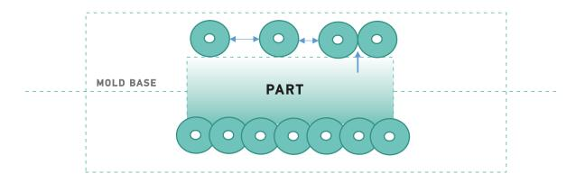
Cooling channels must be installed correctly, if there are any voids between them, cooling effecting the part would not be balanced. That's why warpage issue risk takes place.
